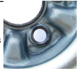
This is a condition that occurs over time. A contributing factor is tightening the wheels down too tightly. The **Ford manual recommends 65-70** foot pounds of torque. It is not uncommon for tire shops to tighten them to 100 foot pounds of torque.
